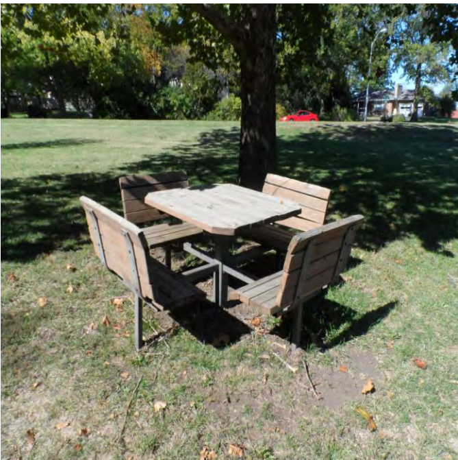
Image 3: Small picnic table that is not accessible and does not have an accessible route to it.
